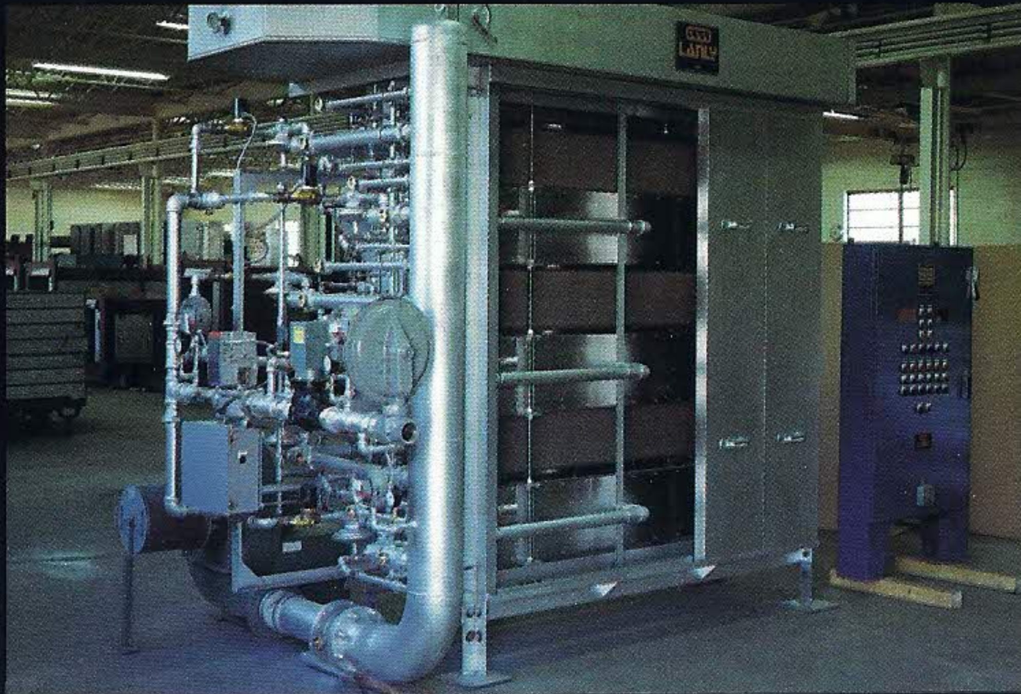
Gas Fired Radiant Predryer
