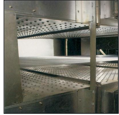
Radius Port ducts above and below yarn ensures uniform, efficient drying
