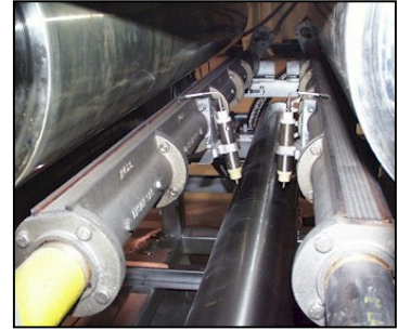
Wide burner faces and large diameter rolls provide sufficient dwell time to ensure quality singeing
